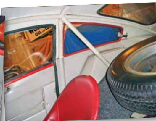
Current interior, showing door panel, carpet, seat, and the vinyl covering of interior tubing.
