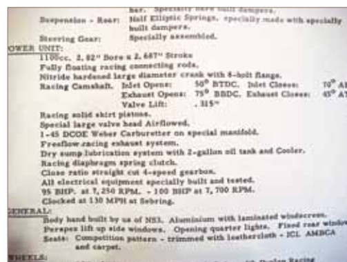
Detail of DHMC spec sheet; rear suspension noted with half elliptic springs.
