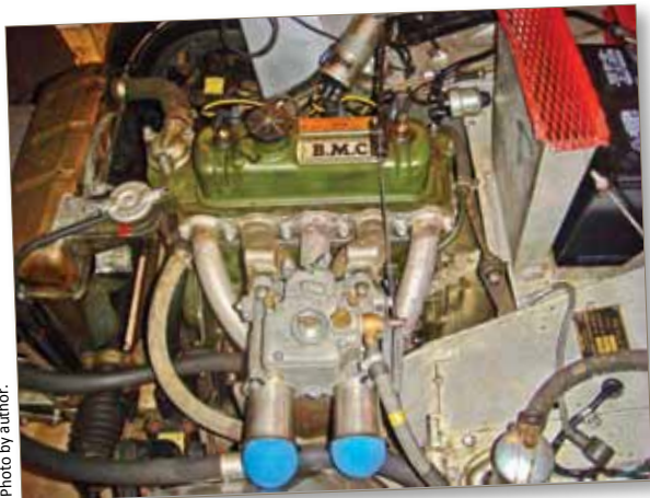
The engine bay showing the Weber carb and dry sump oil reservoir at lower right.
