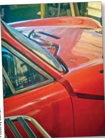
The bonnet cut line showing unusual configuration about windscreen wiper posts.
